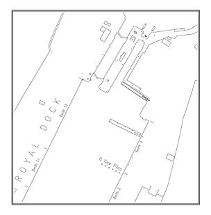
6 piles will be installed approximately 75m South of the current pontoon on berth number 1. The outermost pile will be positioned 45m into the Dock and will be lit with two fixed red navigation lights positioned vertically.
